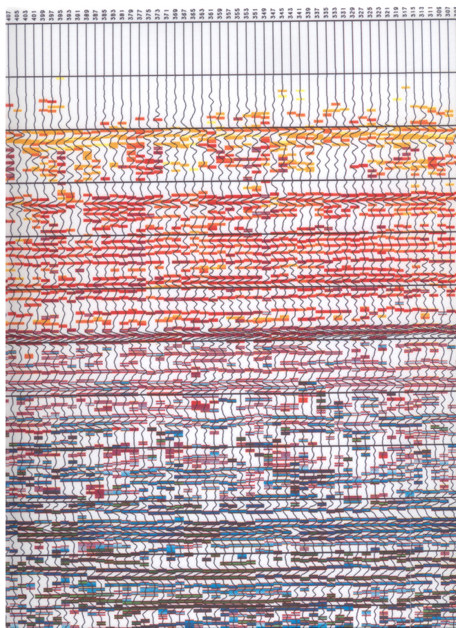
Figure 3. A stacking velocity display with the color boxes representing the velocity.
